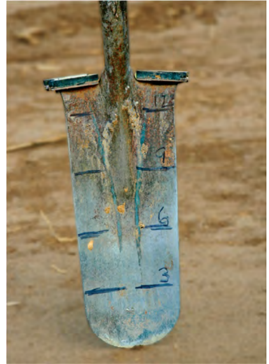
Figure 3-27 | A shovel can be used to determine depth to compaction
