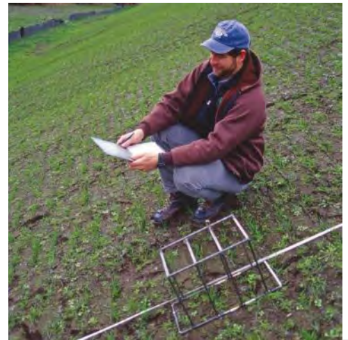
Figure 6-4 | Fixed frame for measuring soil cover
