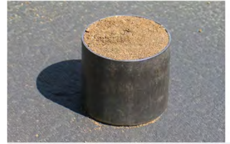
Figure 3-26 / A soil core is used to assess soil compaction
