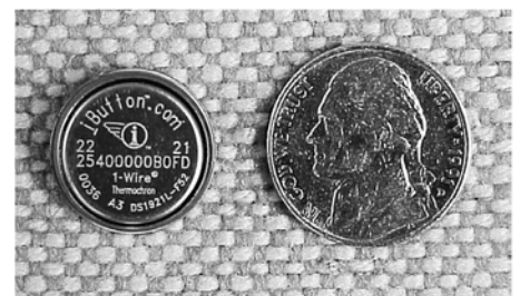
Figure 3-33 | Temperature recording device
