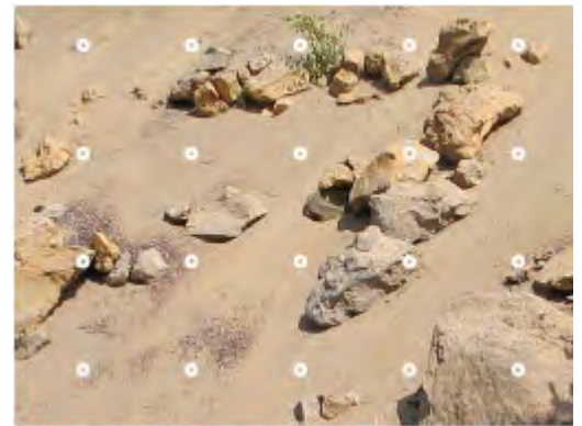
Figure 3-22 | Estimating rock fragment content from roadcuts
