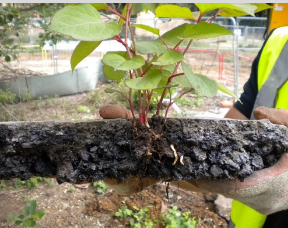
Japanese knotweed roots growing through pavement.
